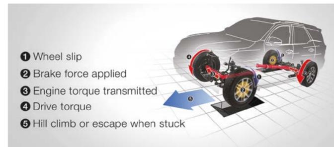
Active Traction Control (A-TRC)\*: When driving off-road or in slippery conditions, A-TRC applies brake pressure to prevent wheels from spinning during acceleration.
