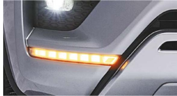
The angular headlamp design has been realised by separating the turn signal/position lamp from the headlamp.
