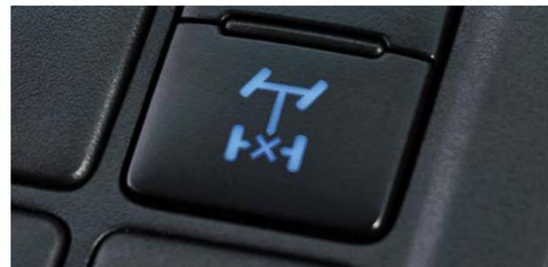
The Rear Differential Lock system helps secure traction when driving in muddy terrain, or in the unlikely situation when the vehicle is stuck. The vehicle is equipped with a solenoid switch differential lock system.
