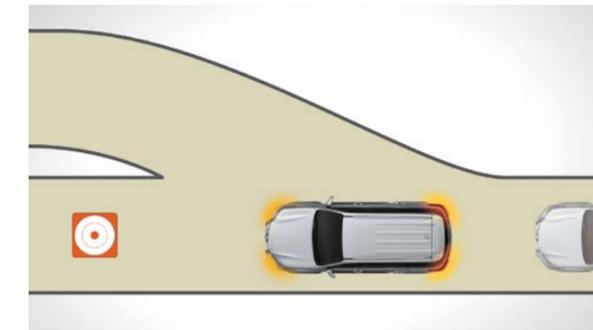
The Emergency Brake Signal automatically activates the brake and hazard warning lights when it detects an emergency stop situation after 60km/h. The lights blink rapidly 3 times to warn following vehicles that the car is stopping abruptly, reducing the risk of a collision.
