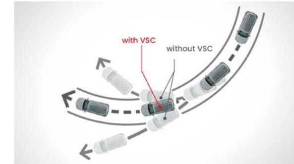
Vehicle Stability Control (VSC) to keep you in control and the vehicle pointing straight when on slippery surfaces by individually applying braking to each tyre where necessary.
