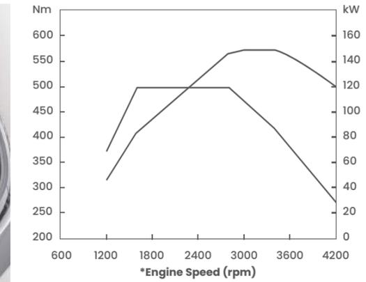
The New Generation 2.8-liter Diesel engine (1GD-FTV) has been optimally tuned for higher output and enhanced fuel economy. Refinements have been made to the Variable Nozzle Turbocharger and Intercooler, which contribute to both higher power and torque output with better fuel economy. The result - a prodigious +20kW Power output improvement and +50Nm Torque improvement from the previous generation engine.
