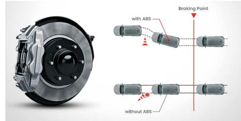
Anti-lock Braking System (ABS), whereby excess brake pressure is modulated to allow for continued tyre rotation under extreme braking conditions, where excessive pressure would ordinarily lock the brakes and induce a skid, eliminating the ability to turn and prolonging the braking distance and possibly leading to a loss of control.
