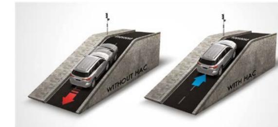
Hill-Assist Control (HAC), so that you don't need to worry about rolling back when pulling off from a sharp incline.
